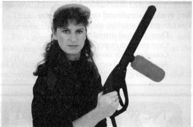
This Foaming Lance applies detergents evenly and quickly.
